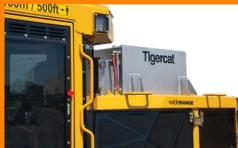
Herbicide and water tank are made of stainless steel to reduce the risk of corrosion.
