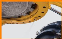
The spray system nozzle located behind the saw Components are blade on the rear skirt housing provides an effective within the carrier. and even spray pattern.
