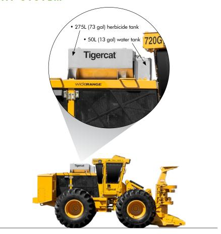
The Tigercat coppice spray system is available for both Tigercat wheel and track feller bunchers.
