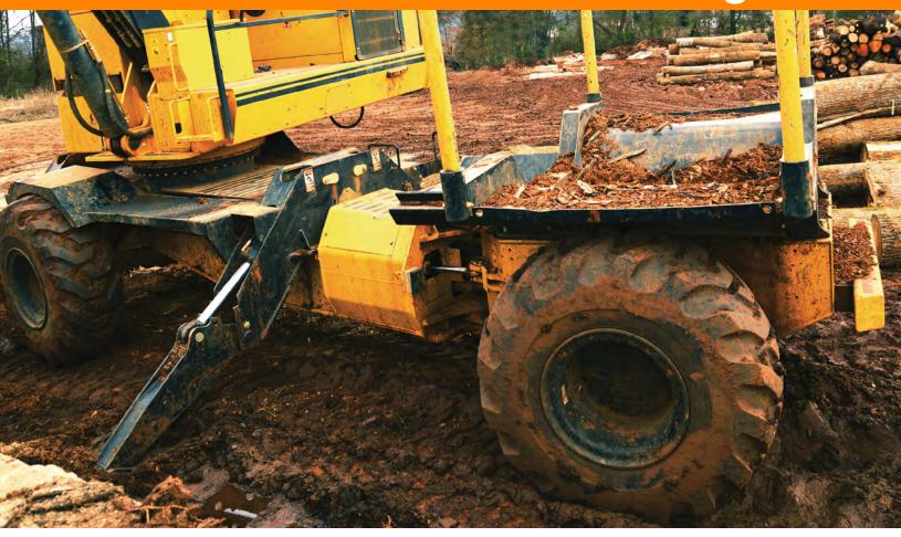
The AC16 articulating carrier is designed and built for mill yard duties with powerful tractive effort and durable construction throughout. Tigercat's WideRange® drive provides quick travel speeds without the need to shift gears.
