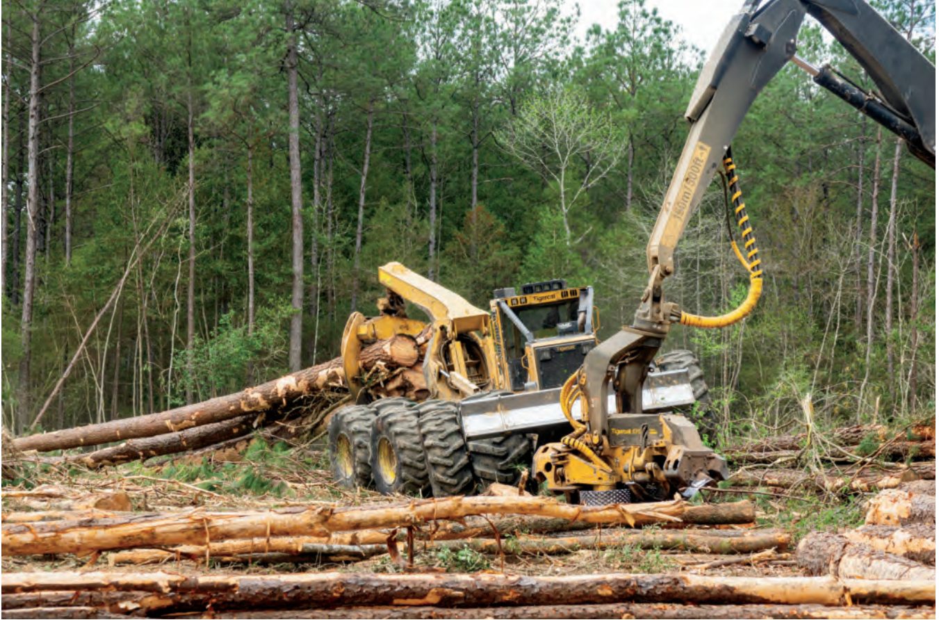
One buncher, one six-wheel skidder and a processor makes for a balanced harvesting system in most situations.
