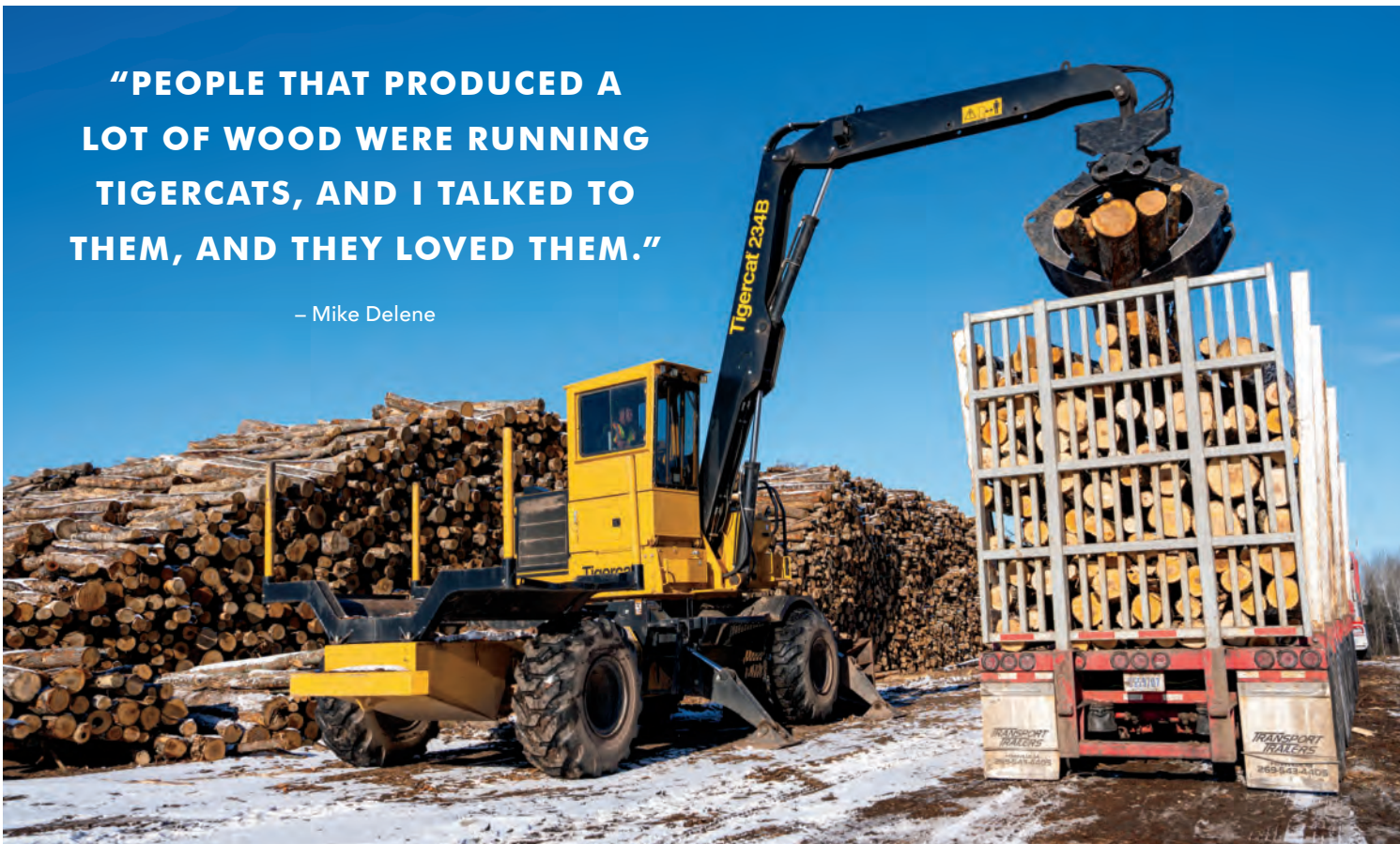
The AC16 articulating carrier is designed and built for woodyard duties with powerful tractive effort and durable construction throughout. Tigercat's WideRANGE drive provides quick travel speeds without the need to shift gears.
