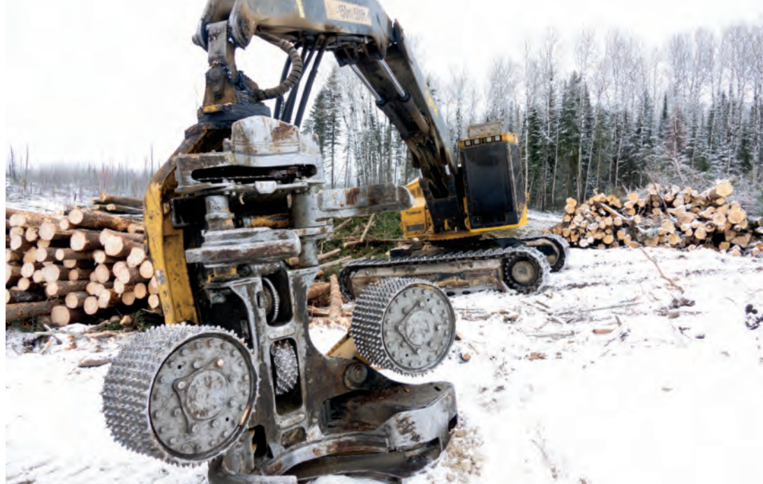
Brander's oldest Tigercat 575 head has 38,000 operating hours. It is double shifted throughout the season.
