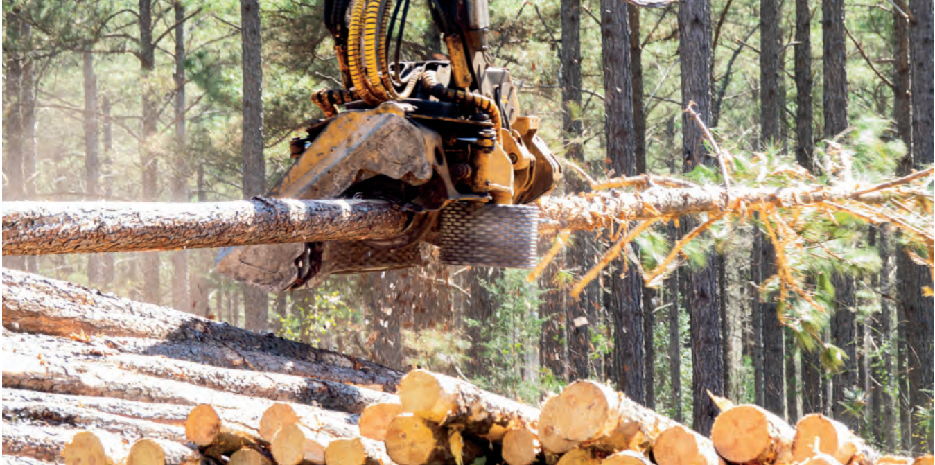
No guesswork, no tape measures. The processor accurately measures diameters over the entire length of the log.
