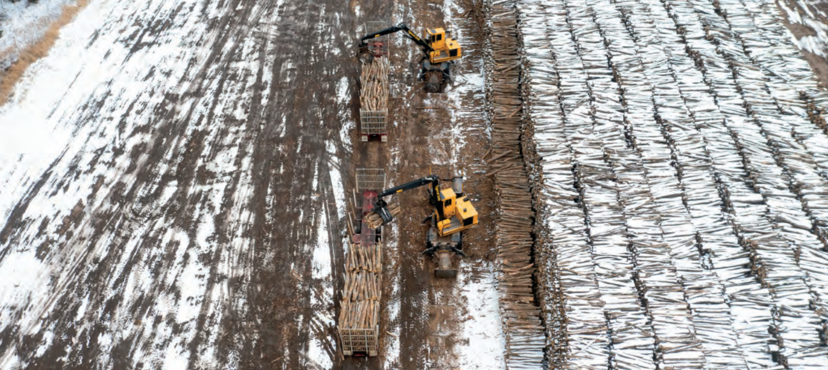
The Tigercat loaders are an excellent choice for the woodyard. With efficient load sensing hydraulics and a unique energy recovery swing system, Mike says that fuel economy is outstanding.
