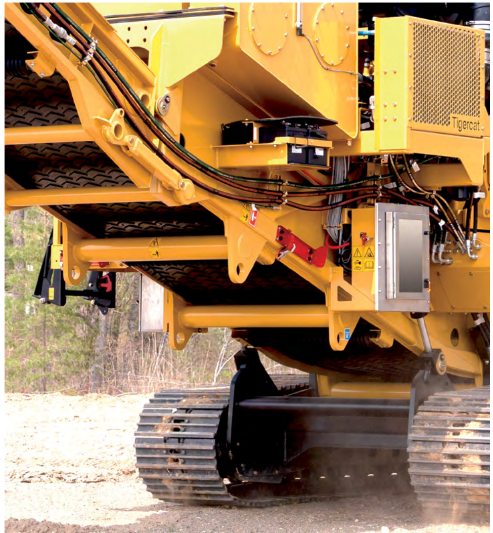
Toolbox that hydraulically raises and lowers.
