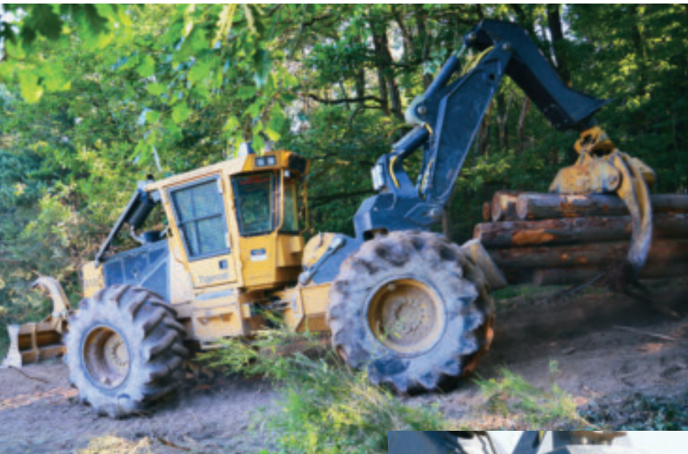
Tigercat 610C skidder fitted with a swing boom designed and manufactured by Belgium based Charlier Engineering.
