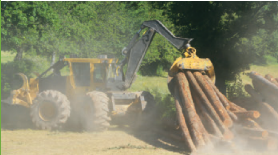
The swing boom makes it quicker and easier to build high decks when space is limited.
