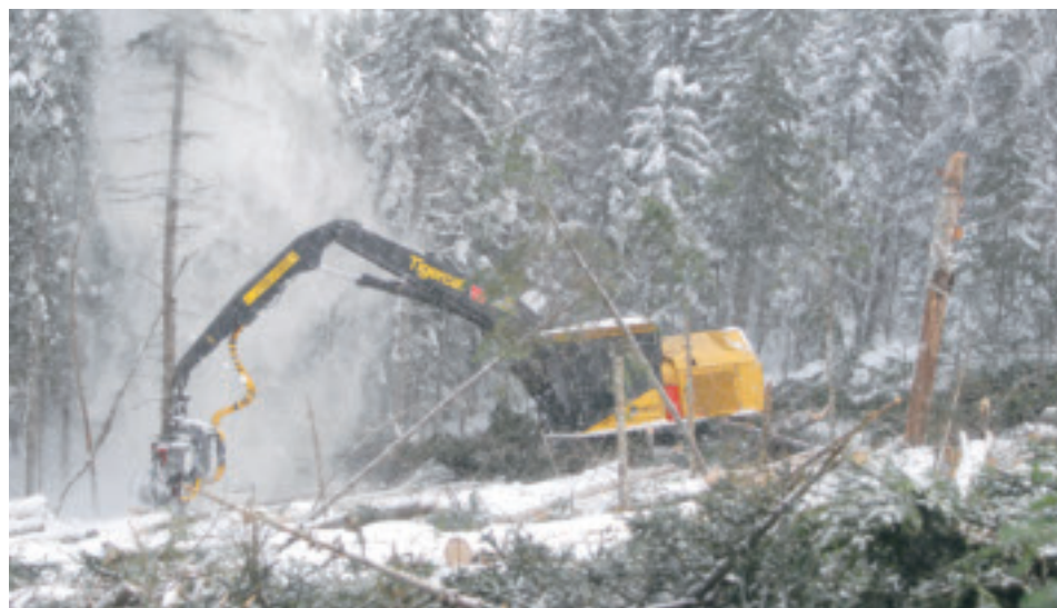
Tigercat H855C track harvester laying wood for the 1085B forwarder.
