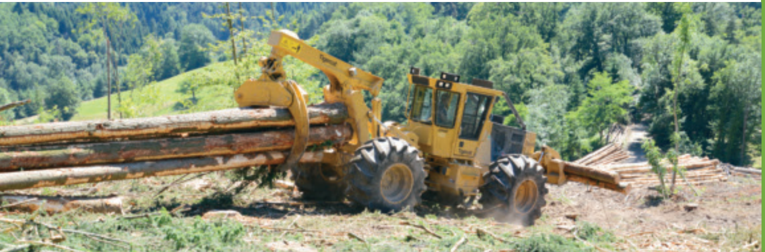
The 610E grapple skidder equipped with front blade grapples for sorting logs and transporting shortwood.
