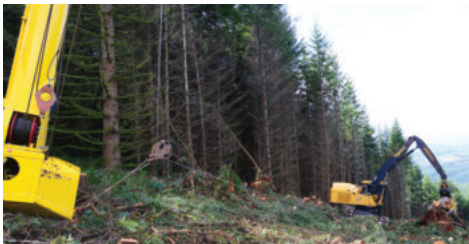
The operator controls the winch as he descends or ascends the slope, preventing sliding and allowing for downhill felling.
