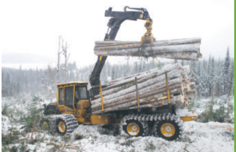
The 1085B forwarder with the Tigercat F195T85 crane, Tigercat FG43 grapple and low-wide bunk.
